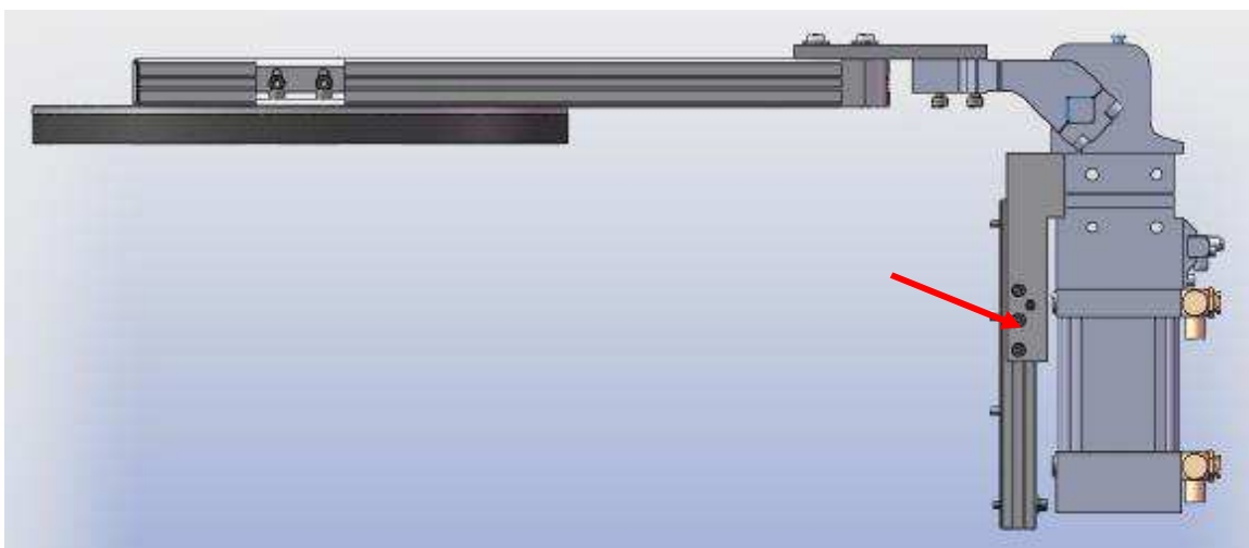
Figure 11: Refasten Actuator Sliding Plate loosening bolts and set screw.
